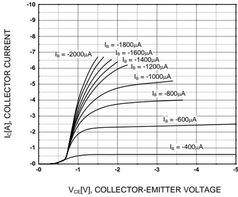
Figure 1. Static Characteristic
